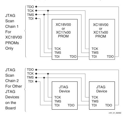
Figure 1: Separate JTAG Scan Chain for the PROMs
