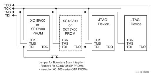
Figure 2: JTAG Scan Chain for PROMs With Jumpers to Maintain Boundary Scan Integrity
