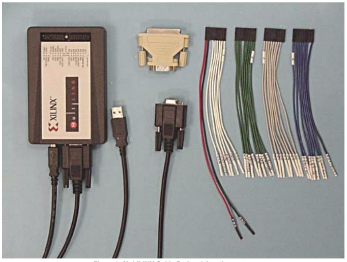
Figure 1: MultiLINX Cable Pod and Attachments
