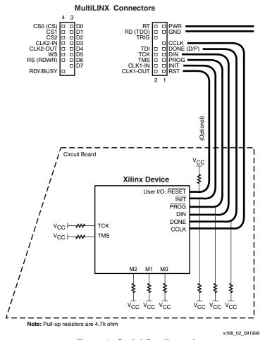
Figure 2: Serial Configuration
