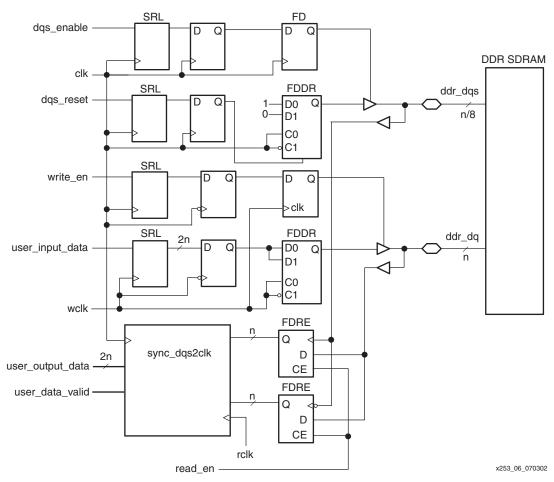
Figure 6: DDR SDRAM Controller Data Path
