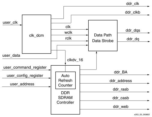
Figure 2: Controller Block Diagram
