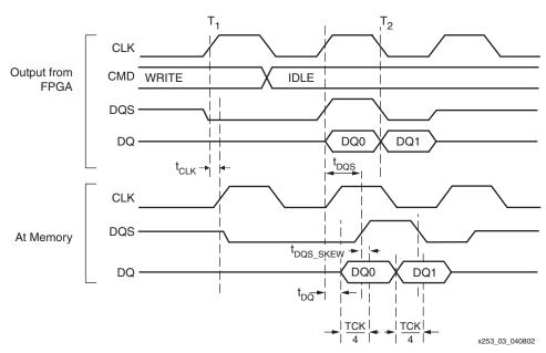
Figure 9: Timing Diagram of Memory Setup And Hold Requirements
