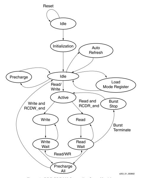
Figure 3: DDR SDRAM Controller State Machine
