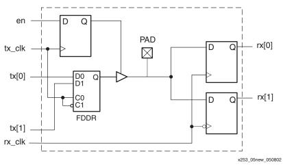
Figure 5: DDR IOB Example Implementation
