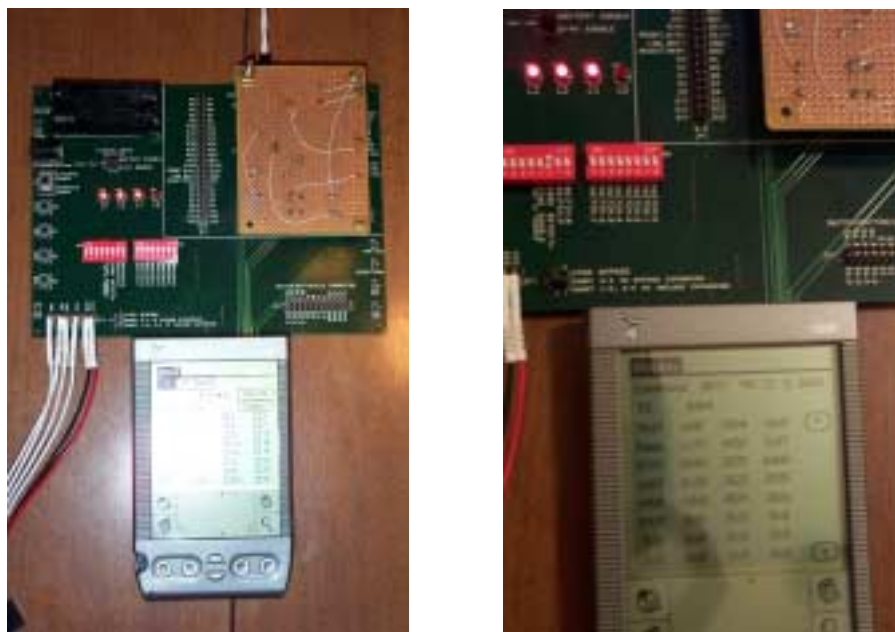
Figure 4: Photos Showing the Interface Board Installed and the Program Running
