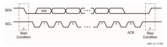
Figure 2: Data Transfer on the I<sup>2</sup>C Bus
