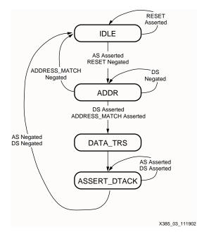
Figure 5: µC Bus Interface State Machine
