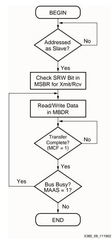
Figure 11: Slave/Transmitter Flow Chart
