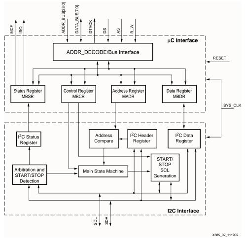
Figure 3: CoolRunner-II I<sup>2</sup>C Controller
