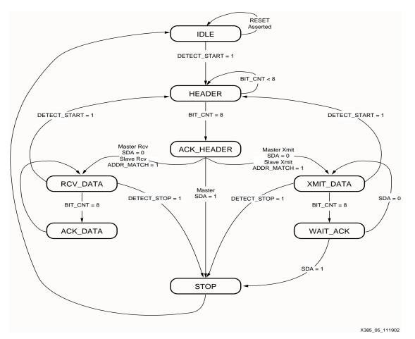
Master to Slave mode if arbitration is lost or if the CoolRunner-II I<sup>2</sup>C Controller is addressed as a Slave.
