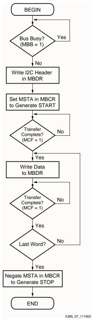
Figure 9: Master Transmit Flow Chart
