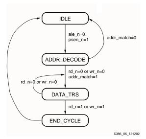
Figure 6: µC Bus Interface State Machine
