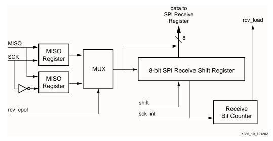
Figure 10: SPI Receive Shift Register and MISO Input Data Registers
