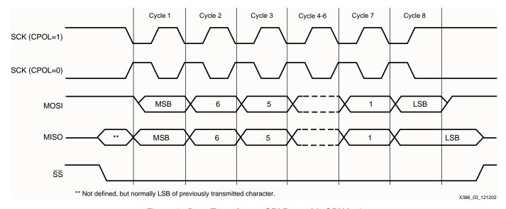
Figure 3: Data Transfer on SPI Bus with CPHA=1
