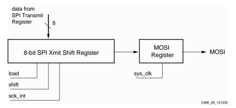
Figure 9: SPI Transmit Shift Register
