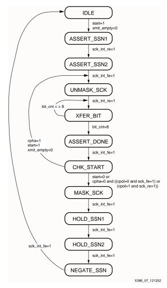
Figure 7: SPI Control State Machine
