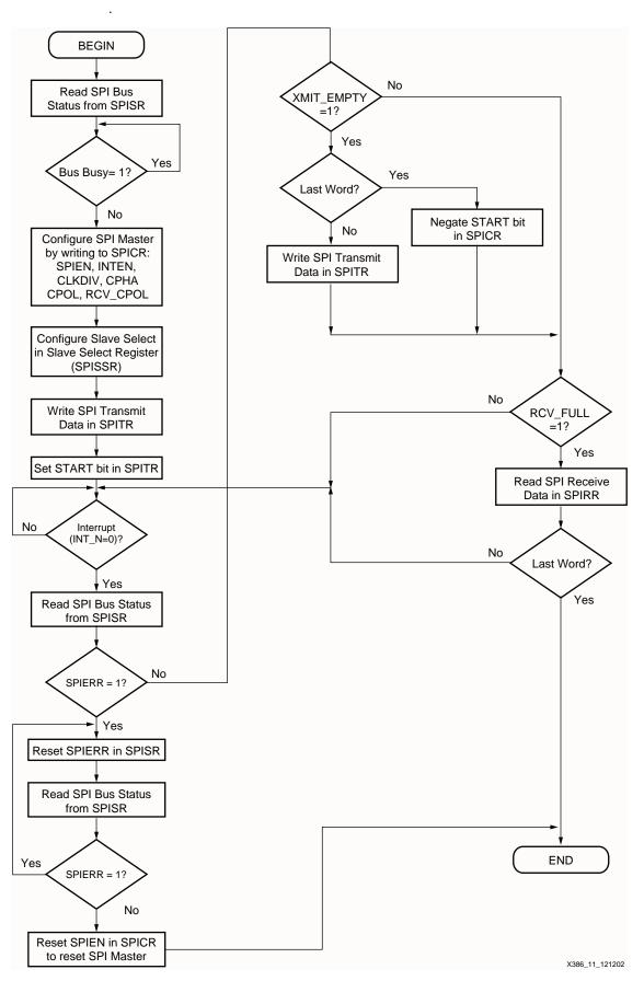
Figure 11: CoolRunner-II SPI Master Transaction Flow Chart
