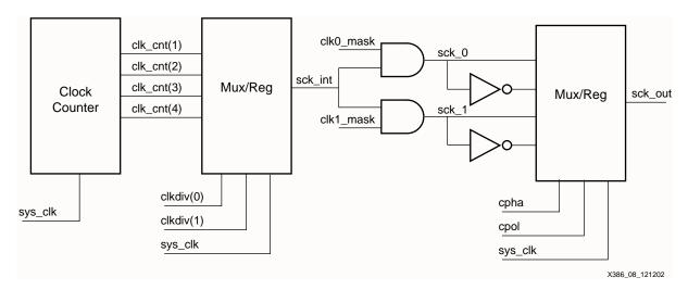
Figure 8: SCK Clock Generation Logic
