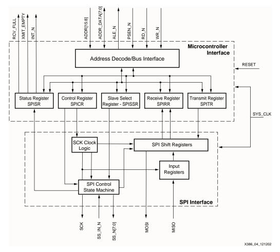
Figure 4: SPI Master Block Diagram
