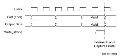
Figure 9: Output Signal Waveform
