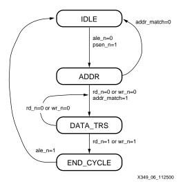
Figure 6: µC Bus Interface State Machine
