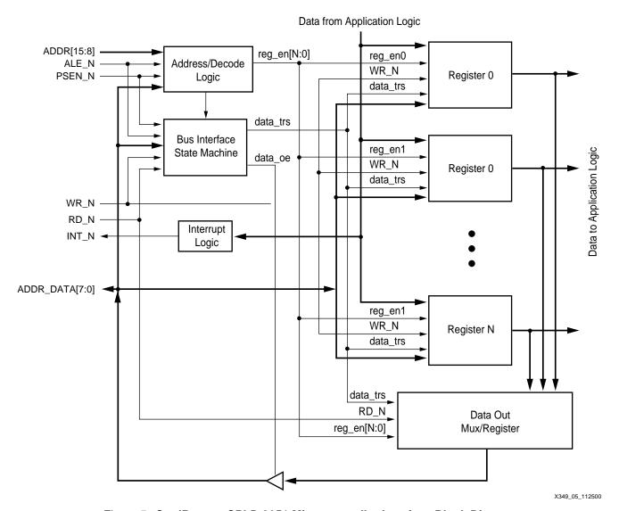
Figure 5: CoolRunner CPLD 8051 Microcontroller Interface Block Diagram
