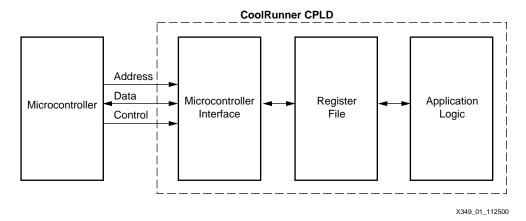
Figure 1: CoolRunner CPLD 8051 Microcontroller Interface
