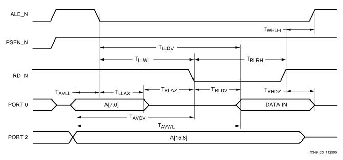
Figure 3: 8051 Microcontroller External Data Memory Read Cycle
