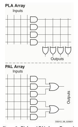
Figure 2: PLA and PAL Array Example
