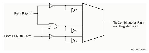
Figure 4: Variable Function Multiplexer
