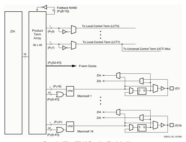
Figure 3: Xilinx XPLA3 Function Block Architecture
