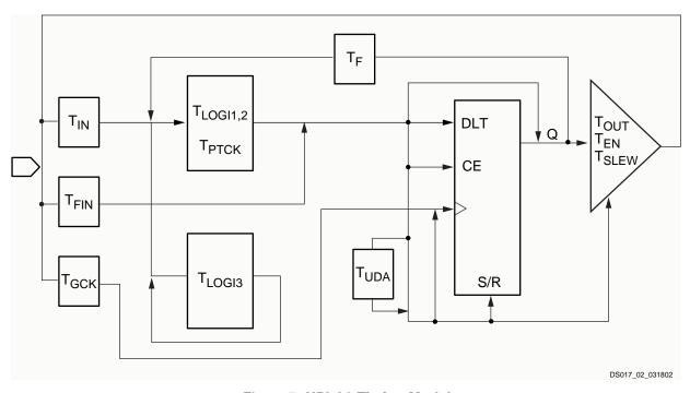
Figure 7: XPLA3 Timing Model
