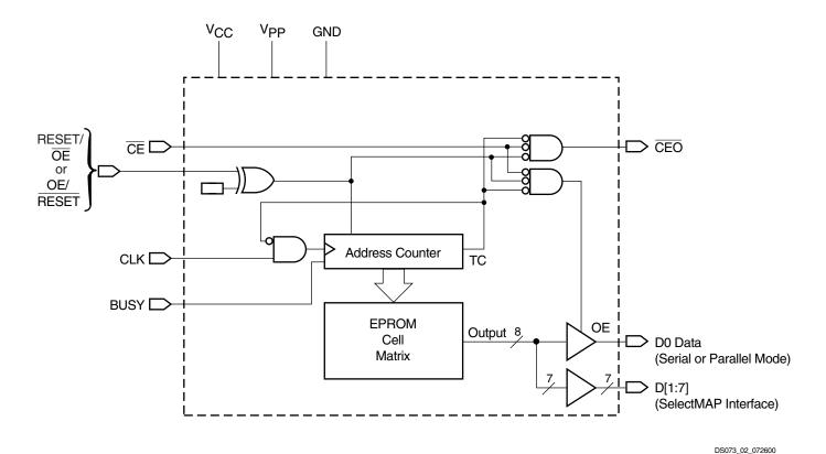
Figure 2: Simplified Block Diagram for XC17V16 and XC17V08 (does not show programming circuit)
