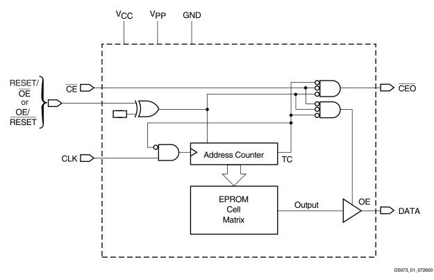
Figure 1: Simplified Block Diagram for XC17V04, XC17V02, and XC17V01 (does not show programming circuit)
