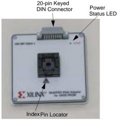
Figure 2: Common Adapter Features
