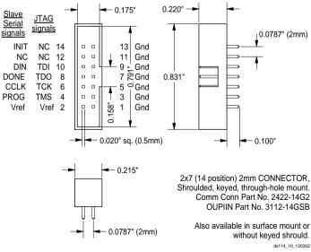
Figure 8: Target Interface 14-Pin Connector Signal Assignments
