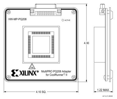
Figure 10: Typical MultiPRO Adapter Dimensions (inches)
