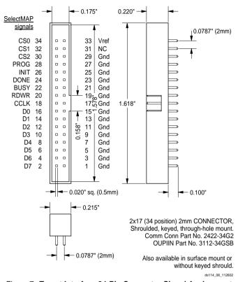
Figure 7: Target Interface 34-Pin Connector Signal Assignments
