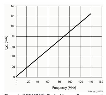
Figure 1: XCR3256XL Typical  $I_{CC}$  vs. Frequency at  $V_{CC}$  = 3.3V, 25°C
