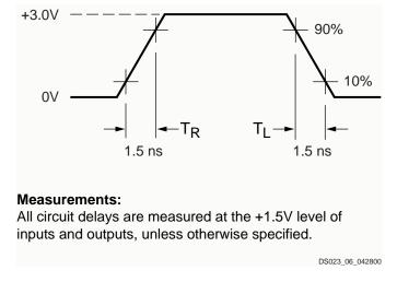
Figure 4: Typical Voltage Waveform
