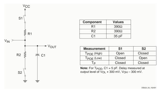
Figure 3: Typical AC Load Circuit
