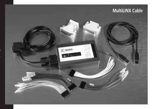
The MultiLINX cable takes advantage of the USB port found on newer PCs. MultiLINX features an adjusting voltage that enables it to talk to system and I/Os operating at 5V, 3.3V, and 2.5V.
