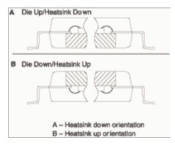
Figure 1: Heatsink Orientation
