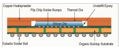
Figure 1: Flip Chip Package
