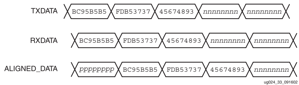
Figure 3-22: RXDATA Aligned Correctly
