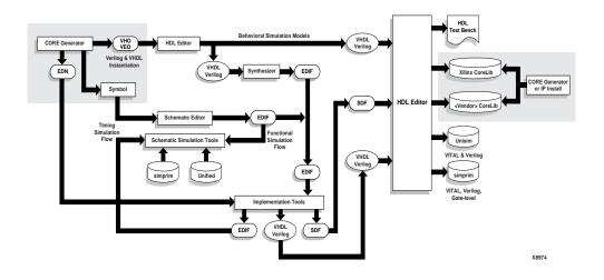
Figure 4-1 CORE Generator Flow Chart
