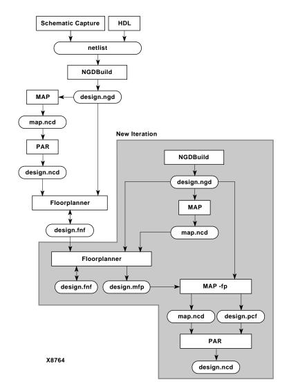
Figure 2-4 Incremental Design Change Design Flow
