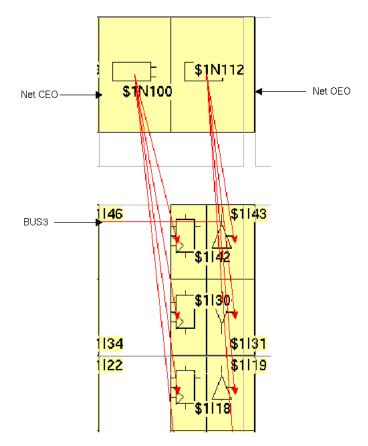
Figure 4-18 Close-up of Aligned Logic Symbols
