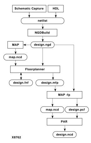
Figure 2-2 Floorplan First Design Flow
