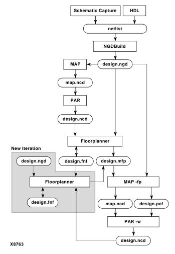
Figure 2-3 Iterative Floorplanning Design Flow
