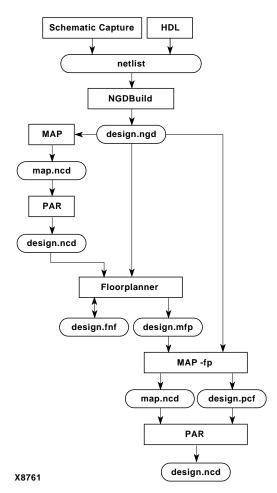
Figure 2-1 PAR Before Floorplanning Design Flow
