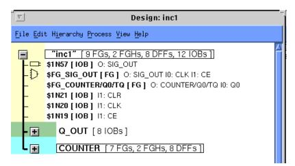
Figure 4-33 Design Hierarchy of New NCD File
