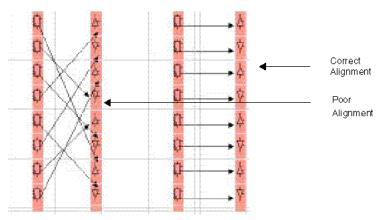
Figure 4-8 Flip-flop/BUFT Alignment Example
