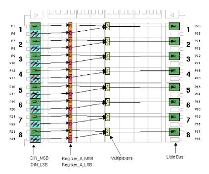
Figure 4-28 Final Placement of Interleave Design
