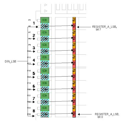
Figure 4-25 DIN\_LSB Placed to Align with REGISTER\_A\_LSB
