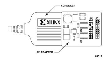
Figure 4-3 3 V Adapter Connected to XChecker Cable
