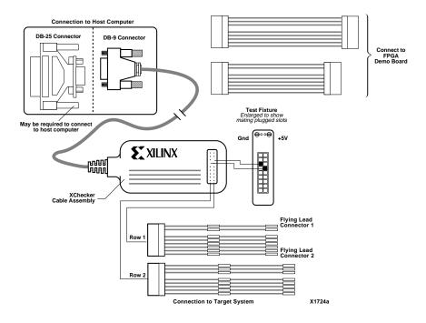
Figure 4-2 XChecker Hardware and Accessories
