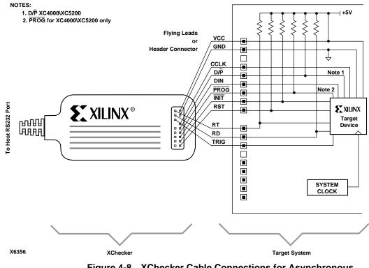
Figure 4-8 XChecker Cable Connections for Asynchronous Debugging
