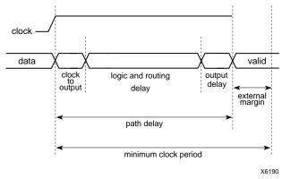
Figure 3-7 Clock-to-Pad Path
