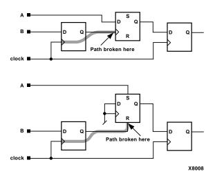
Figure 3-6 Not Propagating Through Asynchronous Set/Reset
