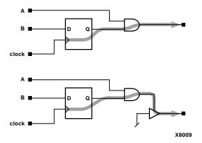
Figure 3-8 Through Tristate Controlled Pads
