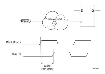
Figure 3-10 Paths Ending at Clock Pin of Flip-Flops
