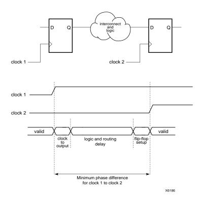
Figure 3-5 Clock-to-Setup Path (Different Clocks)
