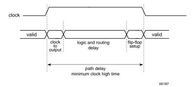
Figure 3-3 Clock-to-Setup Path (Rising to Falling Edge)
