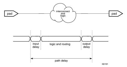
Figure 3-12 Pad-to-Pad Delay
