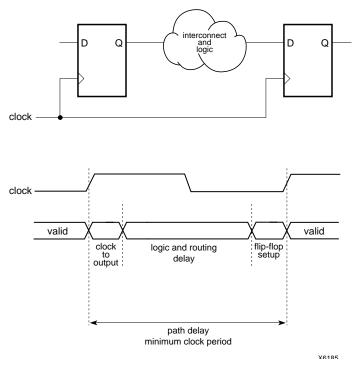
Figure 3-2 Clock-to-Setup Path (Same Clock) with Timing Diagram
