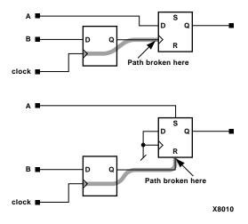
Figure 3-9 Clock-to-Pad Path Broken Through Set/Reset Inputs
