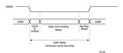
Figure 3-4 Clock-to-Setup Path (Falling to Rising Edge)
