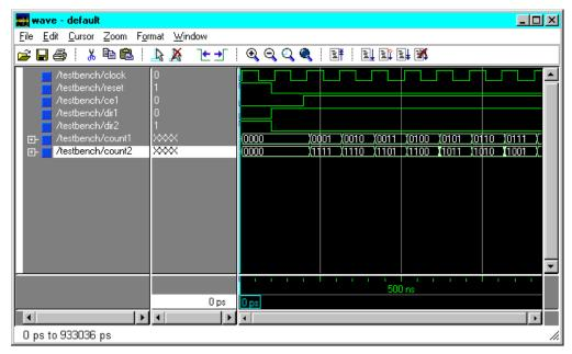
Figure 4-25 Timing Simulation Waveform
