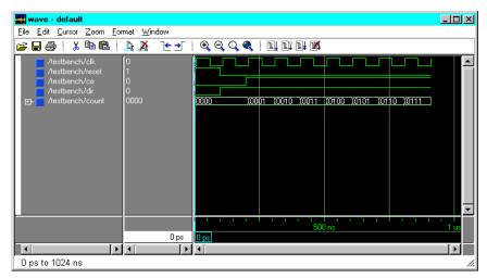
Figure 4-10 Functional Simulation Waveform
