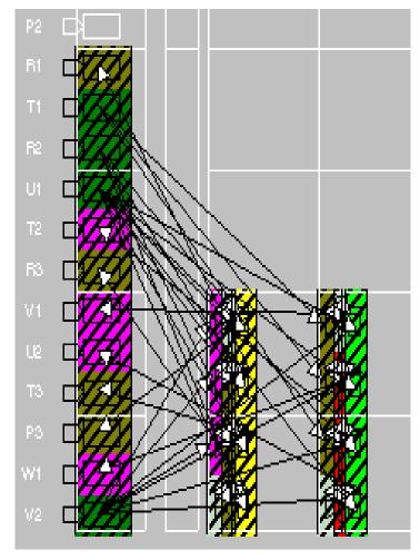
Figure 4-19 I/O Connections in Floorplanner
