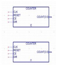
Figure 4-13 Instantiated VHDL Modules
