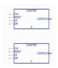
Figure 4-13 Instantiated VHDL Modules
