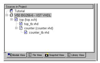
Figure 4-24 Test Bench File in Source Window
