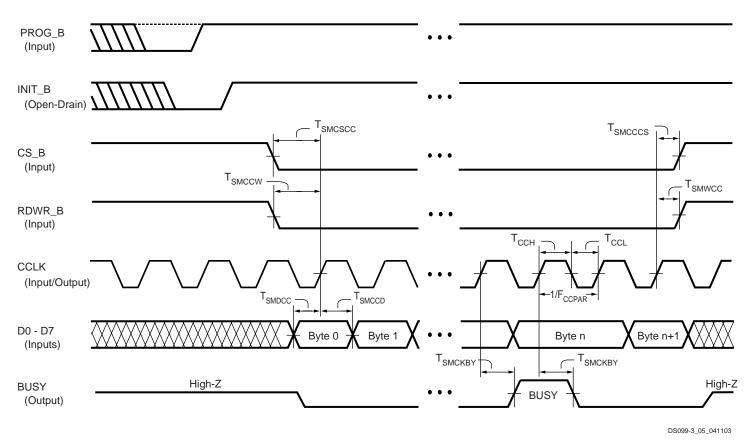
1. In a given CCLK cycle, when RDWR\_B transitions High or Low while holding CS\_B Low, the next rising edge on the CCLK pin will abort configuration.
