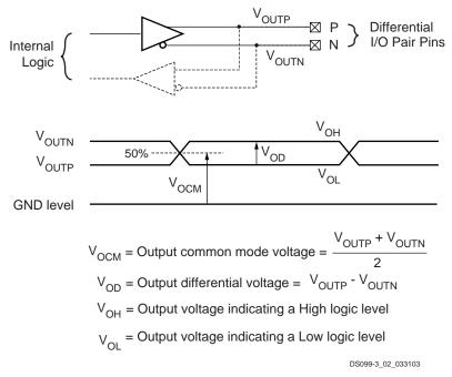
Figure 2: Differential Output Voltages
