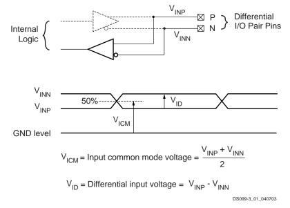
Figure 1: Differential Input Voltages
