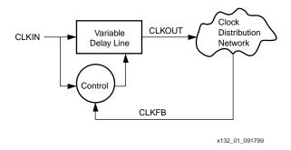
Figure 1: Delay-Locked Loop Block Diagram
