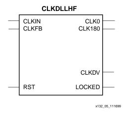
Figure 5: High-frequency DLL Symbol CLKDLLHF
