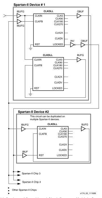
Figure 11: DLL Deskew of Board Level Clock Between Multiple Spartan-II Devices
