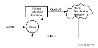
Figure 2: Phase-Locked Loop Block Diagram
