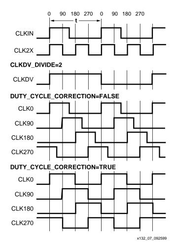
Figure 7: DLL Output Characteristics
