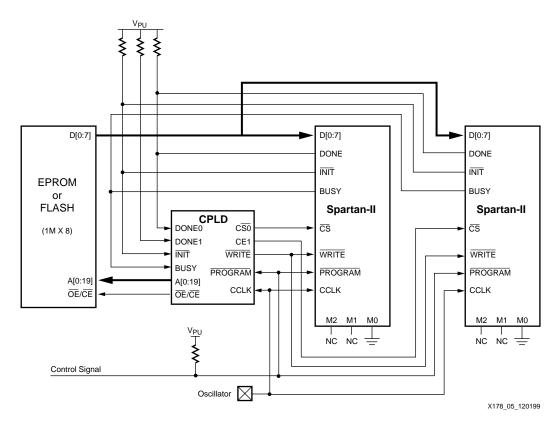
Figure 5: Connecting Multiple FPGAs for Parallel Configuration Chain
