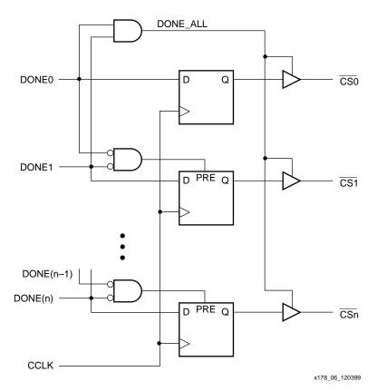
Figure 6: Sequencing FPGA Chip Selects
