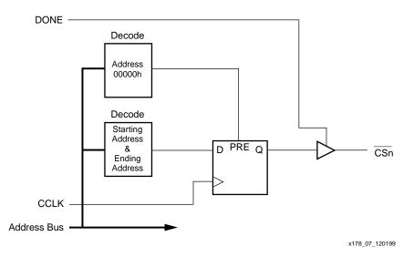
Figure 7: CS Address Decoding
