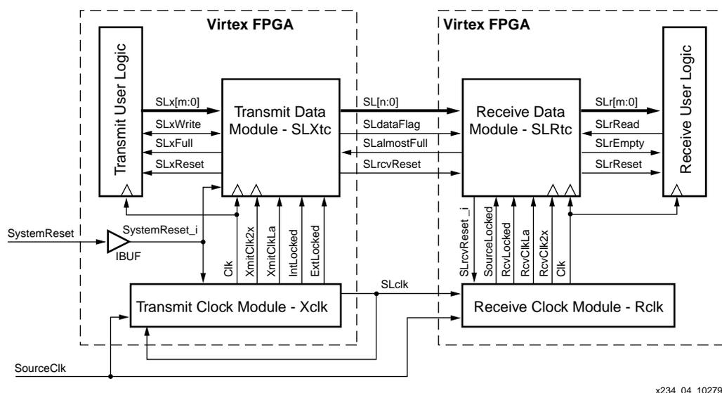
Figure 4: SelectLink Top-Level Modules and Interconnects
