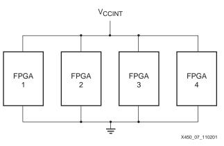
Figure 4: Multiple FPGAs During Power-On
