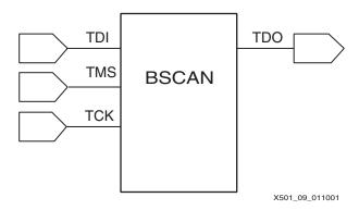
Figure 9: Boundary Scan Spartan-XL Schematic Symbol
