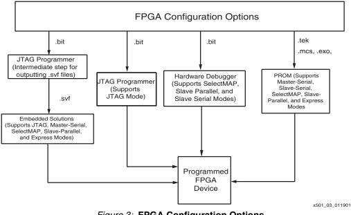
Figure 3: FPGA Configuration Options
