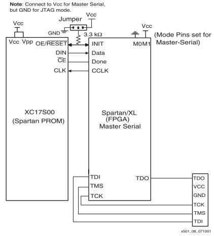
Figure 8: Spartan-XL Master-Serial/JTAG Mode Connections
