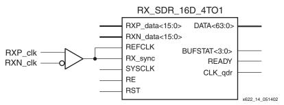
Figure 14: Receiver Clocking with Received Clock
