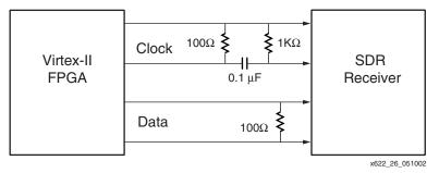
Figure 26: AC Termination and DC Bias Circuit
