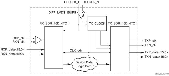
Figure 3: Virtex-II SDR Interface
