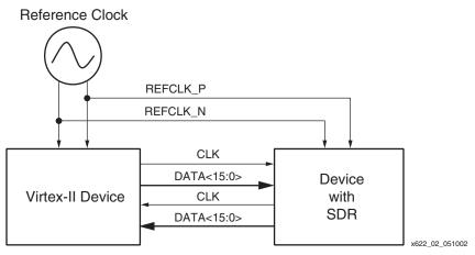
Figure 2: Typical SDR Link System
