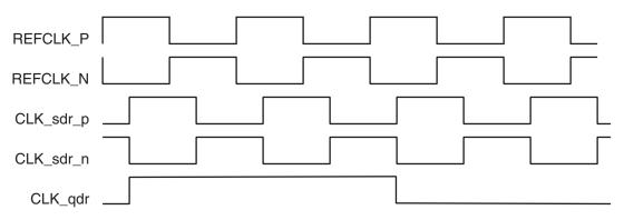
Figure 6: TX\_CLOCK Output Waveforms
