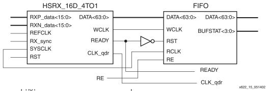
Figure 15: Receiver Block Diagram
