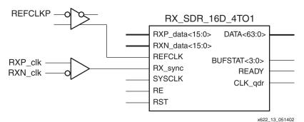
Figure 13: Receiver Clocking with REFCLK
