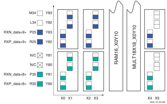
Figure 18: Receive Data Channel Floorplan
