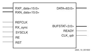
Figure 12: HSRX\_16D\_4TO1 Module
