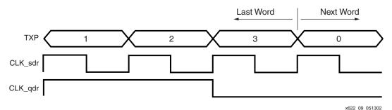
Figure 9: OUTSTAGE\_DATA Output Waveforms
