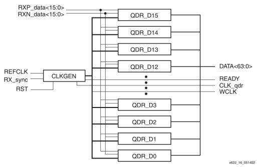
Figure 16: HSRX\_16D\_4TO1 Block Diagram
