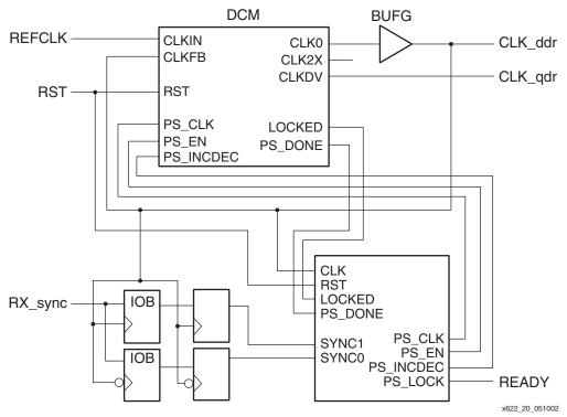
Figure 20: CLKGEN Block Diagram
