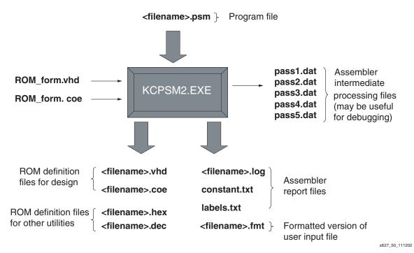
Figure 51: Files Associated with Assembler
