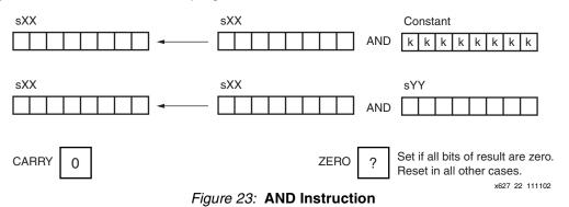
Each AND instruction (Figure 24) must specify the first operand register as "s" followed by two hexadecimal digits. This register also forms the destination for the result. The second operand specifies a second register value in a similar way, or specifies an 8-bit constant using two hexadecimal digits. The assembler supports register naming and constant labels to simplify programming.
