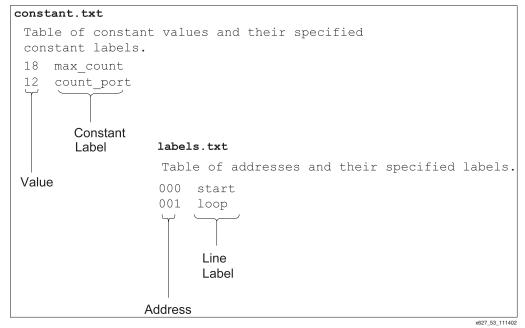
Figure 56: constant.txt and labels.txt Files
