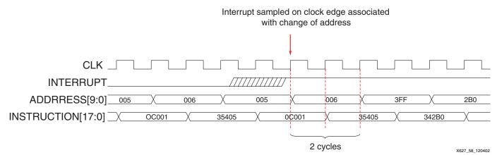
Figure 68: Interrupt Timing
