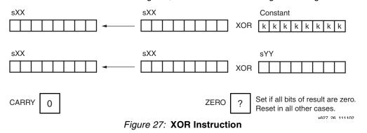
Each XOR instruction (Figure 28) must specify the first operand register as "s" followed by two hexadecimal digits. This register also forms the destination for the result. The second operand must then specify a second register value in a similar way, or specify an 8-bit constant using two hexadecimal digits. The assembler supports register naming and constant labels to simplify programming.
