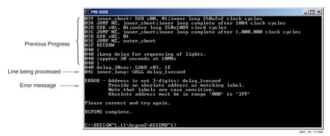
Figure 50: Assembler Error Display
