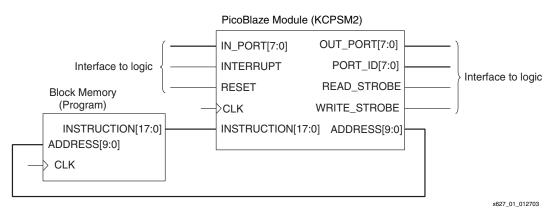
Figure 1: PicoBlaze Module Block Diagram
