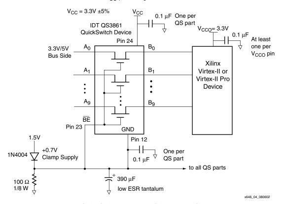
Figure 1: QuickSwitch to Virtex-II/Virtex-II Pro Connection
