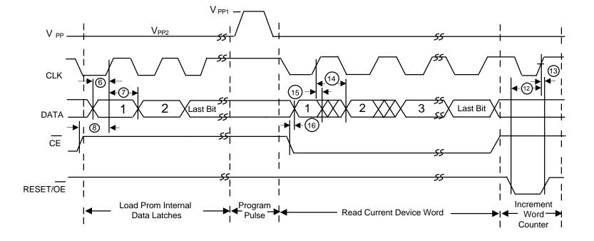
Figure 4. Details Of The Programming Cycle
