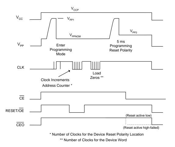
Figure 5. Programming Reset Polarity
