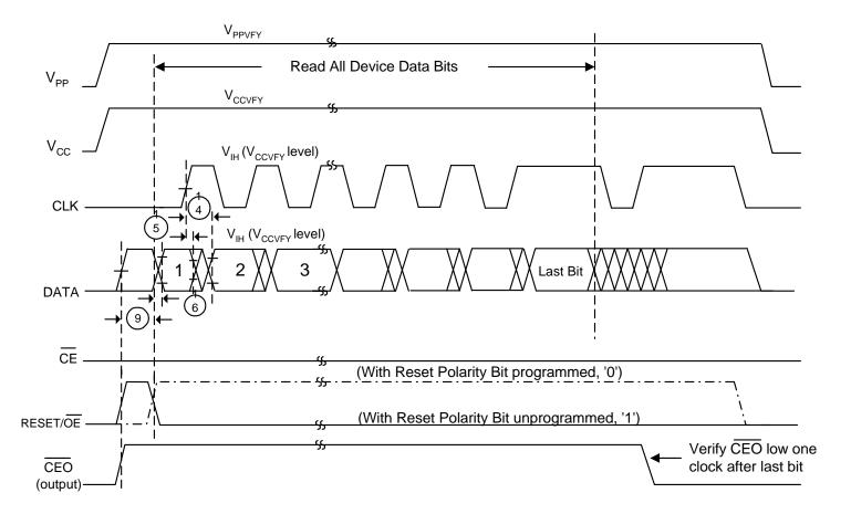
Figure 7. Details Of Verify Cycle
