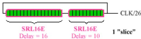
The second stage is a different style than the first, as it must divide the clock enable pulses from the first stage, rather than the clock directly. For this reason, the clock enable input to the SRL16E-based delay is driven.
