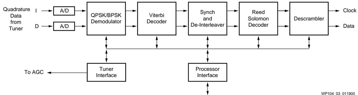
Figure 3: Decoder Block Diagram
