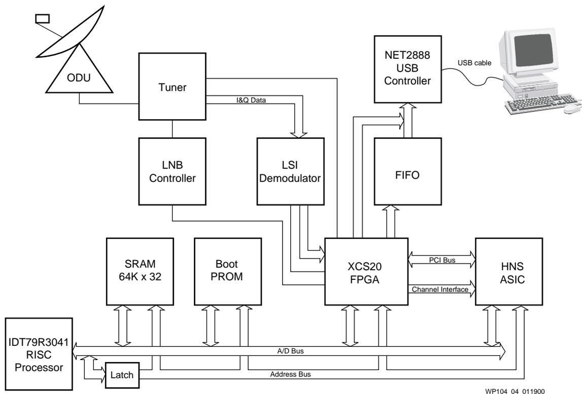
Figure 4: HNS DirecPC®-USB Receiver Block Diagram
