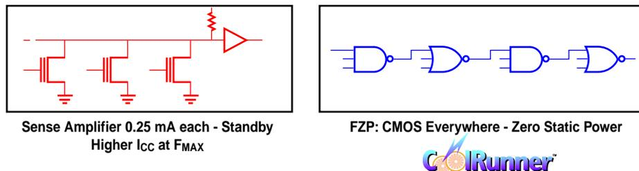
**Figure 2: Sense Amplifier and Fast Zero Power for CoolRunner CPLDs**
