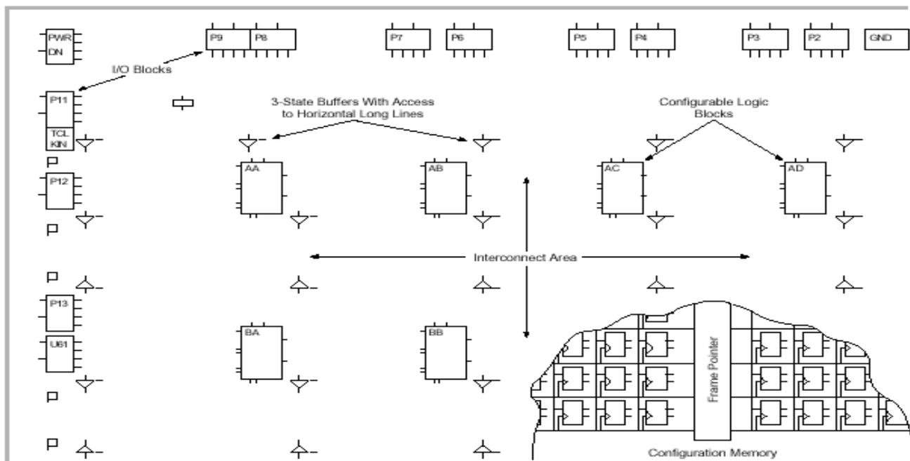
Figure 5: Generic FPGA Architecture
