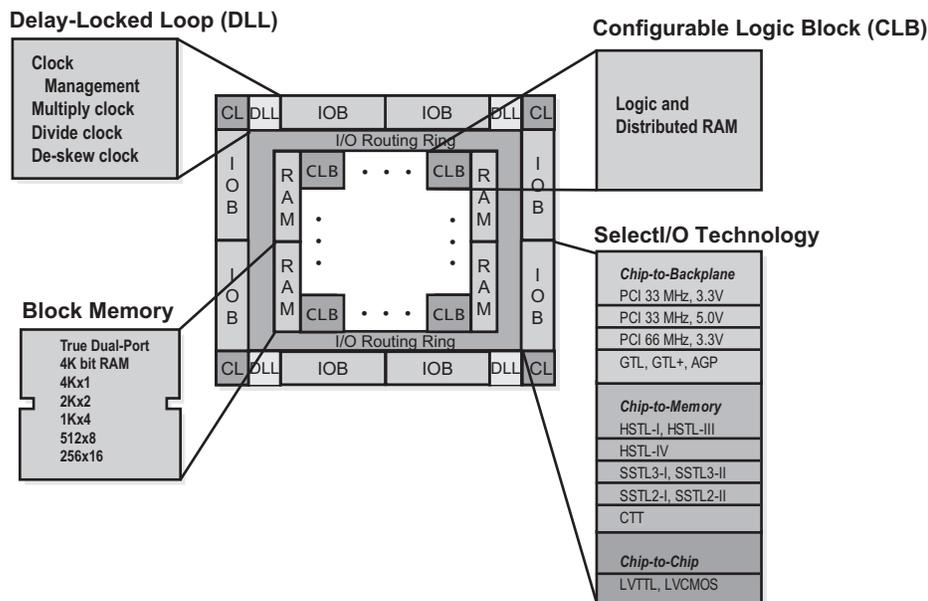
Figure 6: Architecture and Feature Overview of the Spartan-II Family
