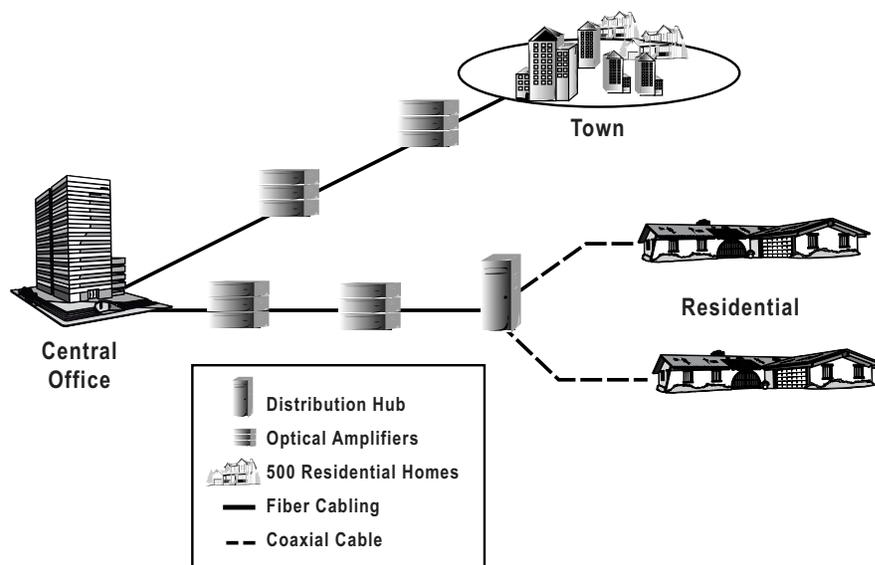
Figure 1: Architecture of a Typical HFC Network
