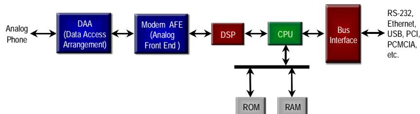
Figure 5: Analog Modem
