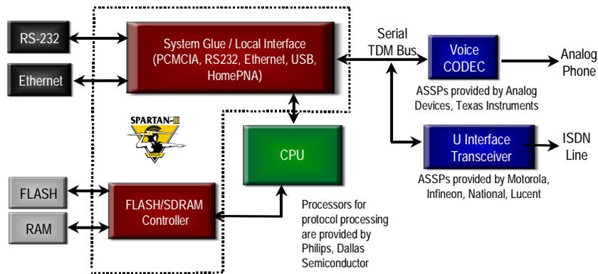
Figure 4: ISDN Modem
