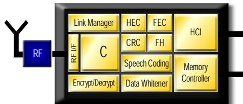
*Figure 5: Bluetooth RF and Baseband Controller*
