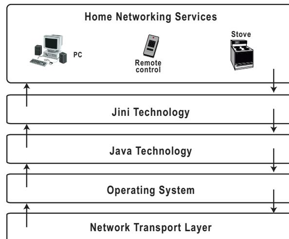
Figure 4: Jini Software Architecture
