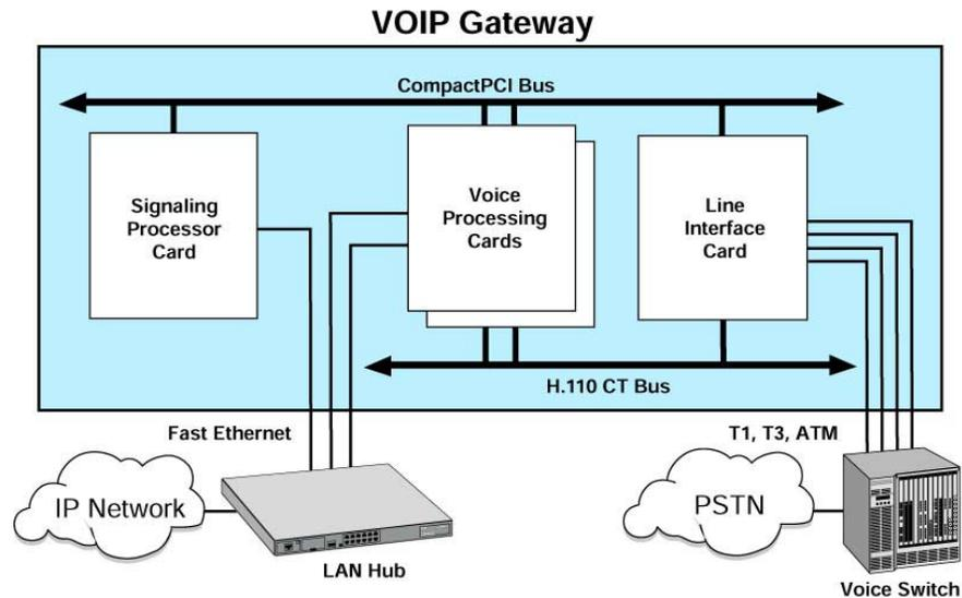
Figure 7: High-Capacity VoIP Gateway Architecture
