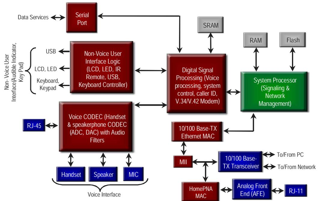
Figure 8: IP Phone Block Diagram
