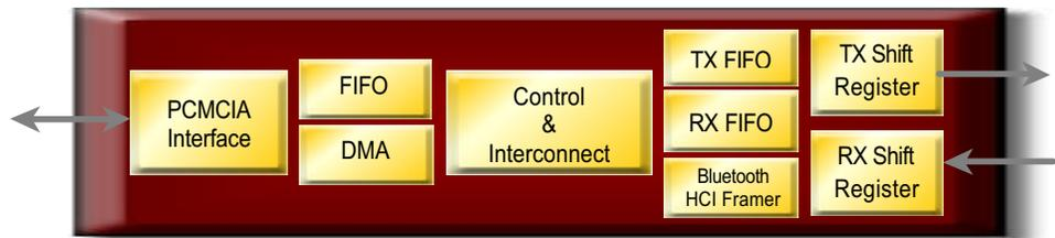
Figure 6: Functional Blocks of High Speed PCMCIA to UART Bridge
