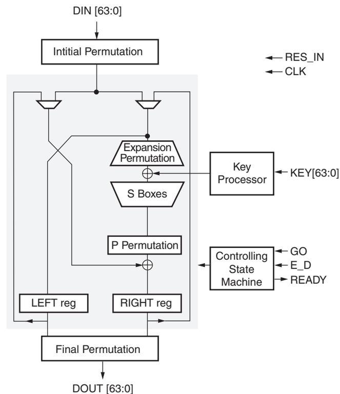
Figure 4: X\_DES Cryptoprocessor Block Diagram (courtesy: Xentec, Inc.)
