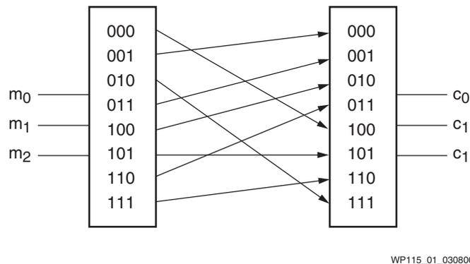
Figure 1: Block Cipher System
