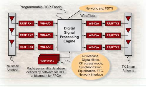
Figure 1 - SDR system diagram
