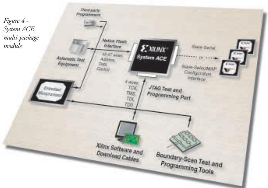
If you want to use a different form factor and mount the components directly on the board, the System ACE Soft Controller IP is available. This pre-engineered solution is identical in functionality to the System ACE MPM solution and you can download the IP free of charge.
