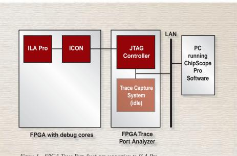
Figure 1 - FPGA Trace Port Analyzer connection to ILA Pro
