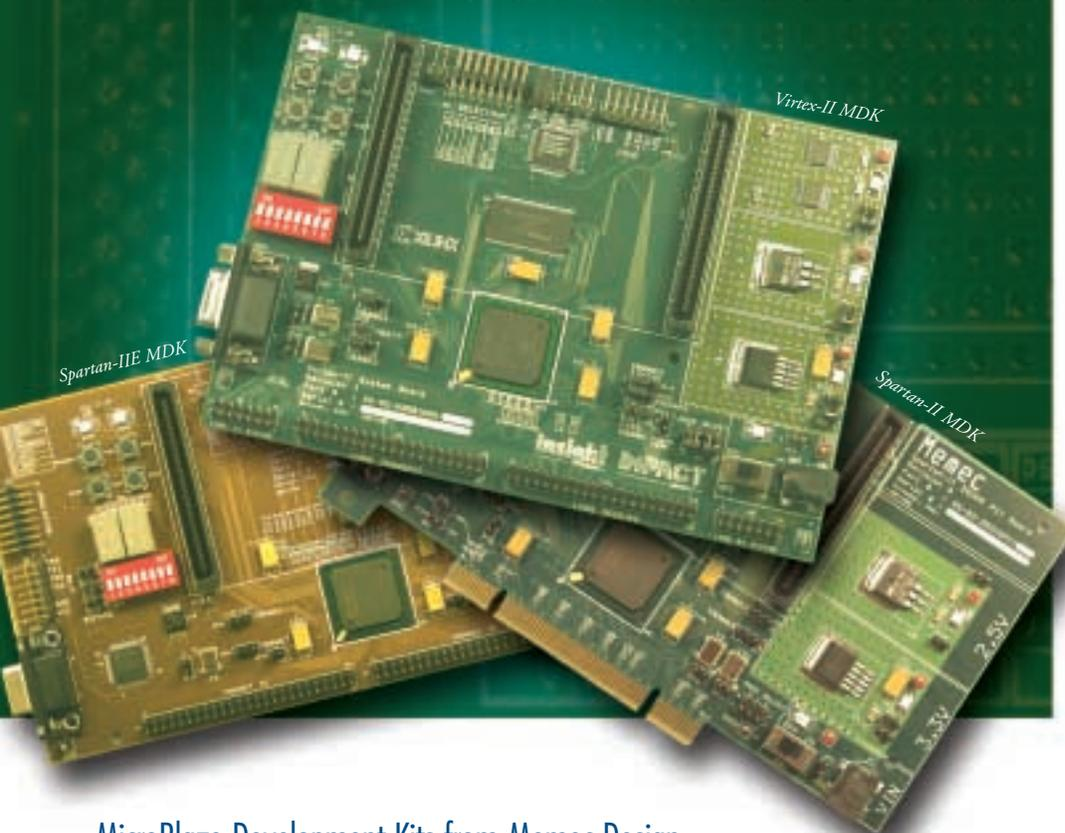
MicroBlaze Development Kits from Memec Design demonstrate the versatility of the MicroBlaze soft processor core in a variety of Xilinx FPGAs.
