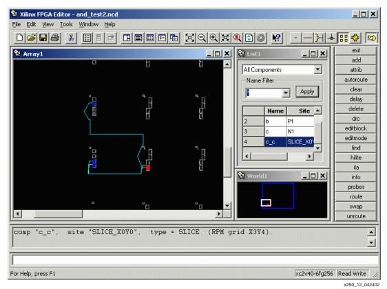
Figure 8: Viewing a Block
