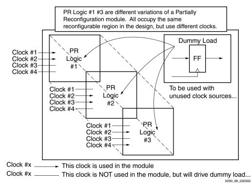
Figure 12: Example of Design Requiring Clock Templates
