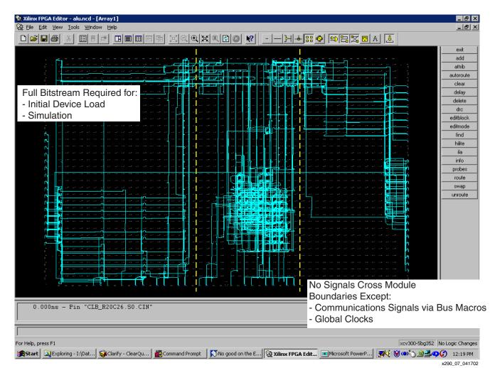
Figure 7: Routed Design After Module Final Assembly
