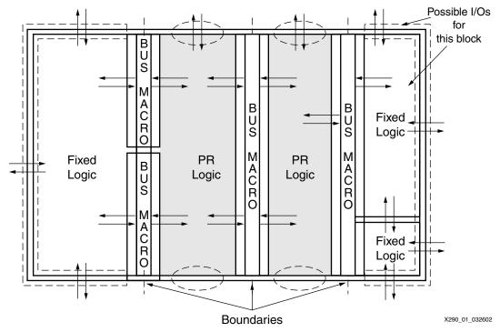
Figure 1: Design Layout with Two Reconfigurable Modules
