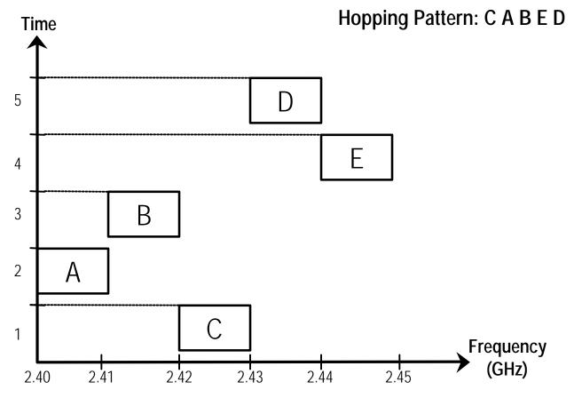
With FH, the Carrier Frequency Changes Periodically - The incoming digital stream is shifted in frequency by an amount determined by a code that spreads the signal power over a wide bandwidth
