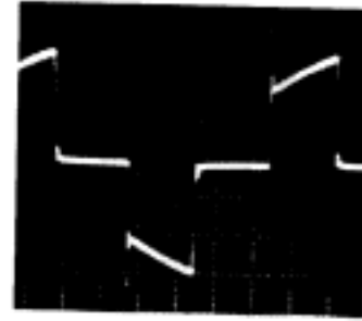
(c) Trans 1次巻線電流波形 (1 A/div, 5 \mu s/div)
