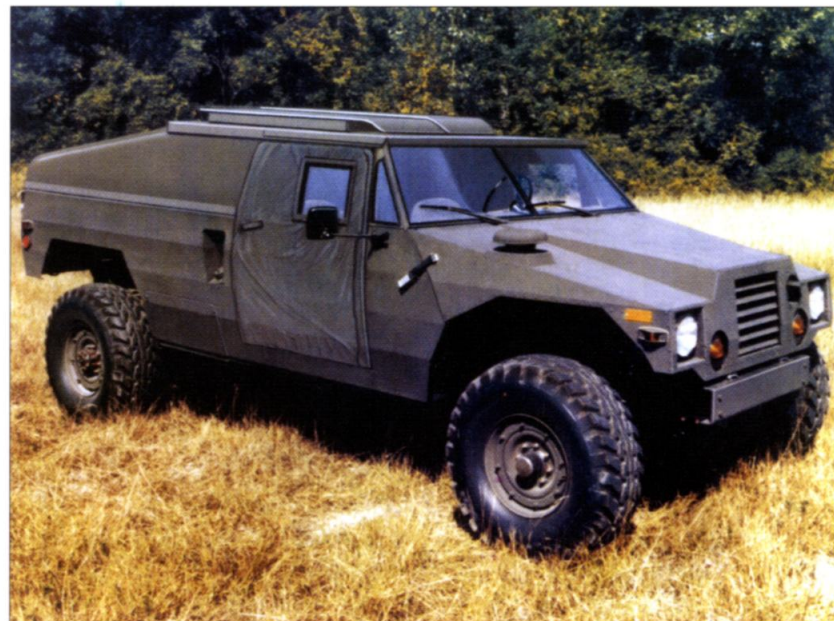
This was the General Dynamics proposal for the armament carrier in the XM966 competition, one of three designs competing for the HMMWV contract. (GDLS)
