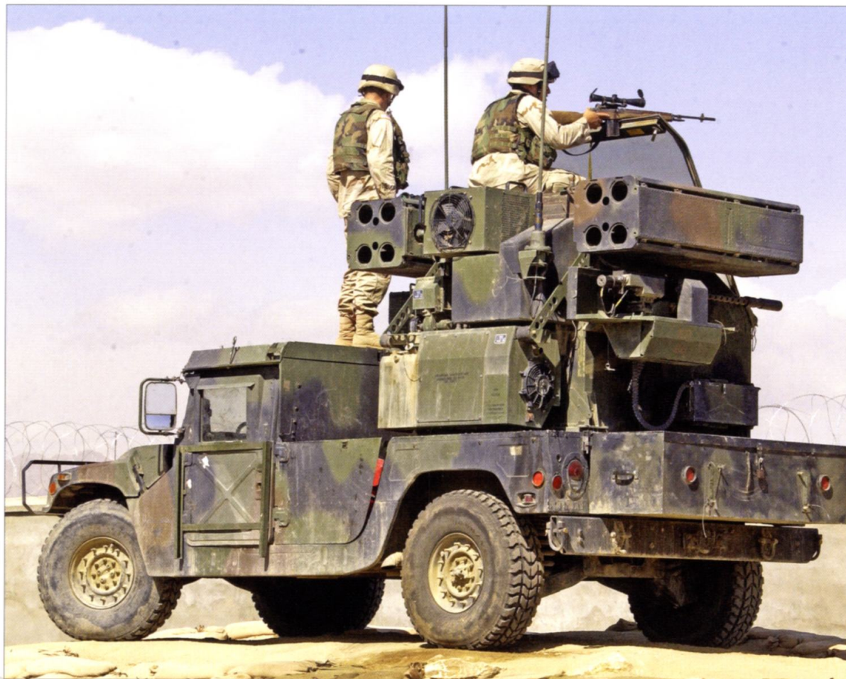
The crew of a PMS Avenger of Battery B, 3/62d Air Defense Artillery maintain a security checkpoint near Ghazni, Afghanistan, in March 2004. The Avenger has proven popular in peacekeeping operations, in spite of the lack of enemy aircraft threats, since its thermal imaging sight is very effective for surveillance day or night at long range. (Sgt Christopher Kaufmann, US Army)
