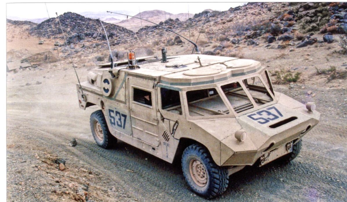
A sheep in wolf's clothing. The Opposing Force units at the US Army National Training Center use Vismod (Visual Modification) HMMWVs to simulate foreign vehicle types, in this case the Soviet/Russian 9P133 (BRDM-2) antitank missile carrier. (Author)
