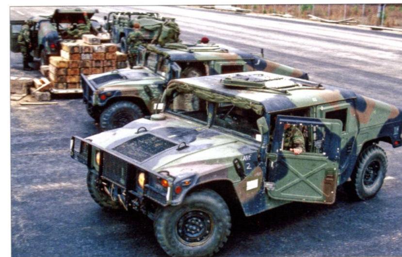
The Army's M1025 armament carrier, like the example seen here from the 82d Airborne Division, can be distinguished from the similar Marine M1043 by the door design. The M1025 with basic armor has the characteristic "X"-pattern door while the Marine M1043 with the heavier "supplemental" armor has a flat door. (Author)
