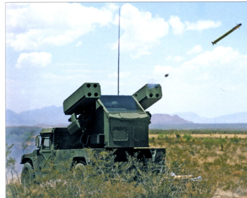
The most successful of the missile HMMWVs has proven to be the PMS Avenger, a combination of the highly successful FIM-92 Stinger short-range air defense missile and the equally successful HMMWV. Each of the pods on either side of the operator's cabin contains four missiles. (Raytheon)
