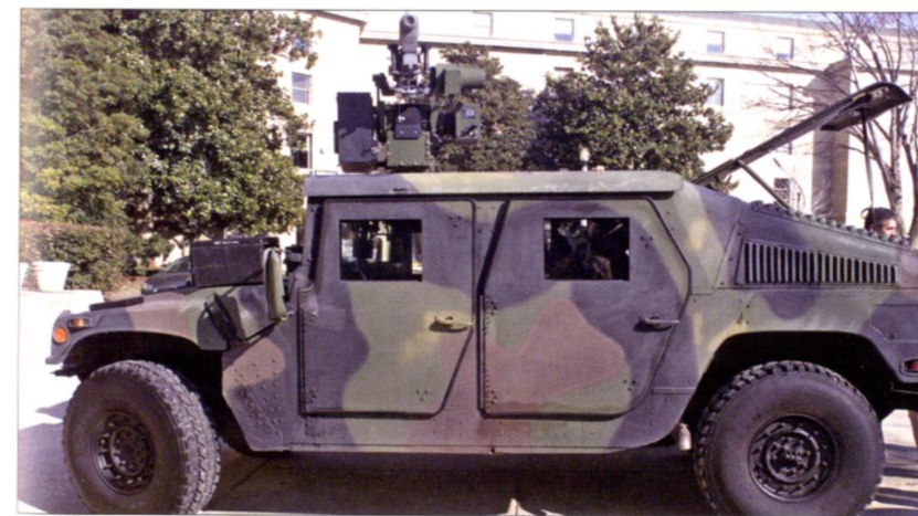
The ultimate package for protecting the HMMWV consists of the Add-On-Armor package as well as the CROWS remote-controlled weapon station, which allows the crew to operate the vehicle weapon from within the vehicle. This vehicle was displayed at the Pentagon in February 2004. (US Army)
