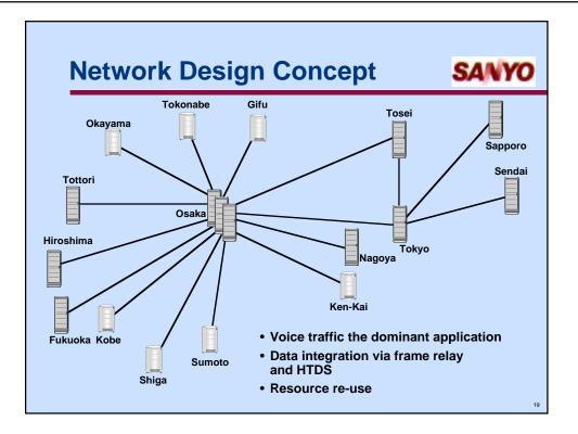
This diagram shows the new backbone network design. The backbone is heavily driven by voice traffic, but also includes the data applications shown on the previous page. The network design criteria for current applications were as follows:
