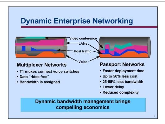
Traditional bandwidth consolidation, using Time Division Multiplexing (TDM) gear and fixed time slot allocation is giving way to new architecture—unified, consolidated, enterprise networks.
